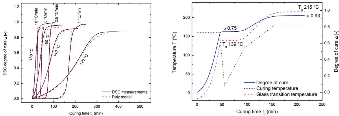
**Figure 2:** Left, Comparison of the Ruiz model to measured DSC data. Right, Example of a simulated curing cycle for a part, where in the second stage the  $T_g$  being above the cure temperature allows free-standing cure.
