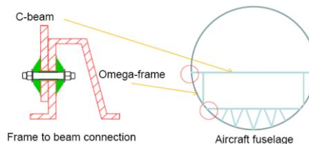
**Figure 1:** *Floor beam to omega frame connection in a fuselage, including reinforcement patches.*
